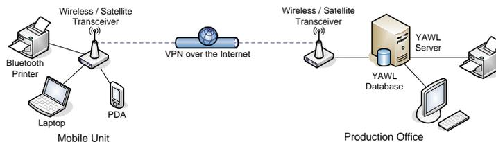
**Fig. 1.** A typical hardware infrastructure for the Film Production Process.
